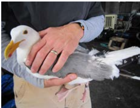
A western gull with a GPS data logger taped to its tail feathers (black object at start of tail). The logger weighs about 20 grams and the gull carries it for 4-6 days. Photo by Emma C. Kelsey 2014.
